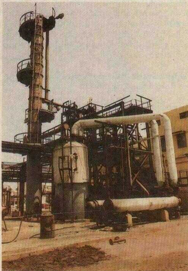
VIII. 1 Purification of Crude Titanium Tetrachloride using indigenous oil.
