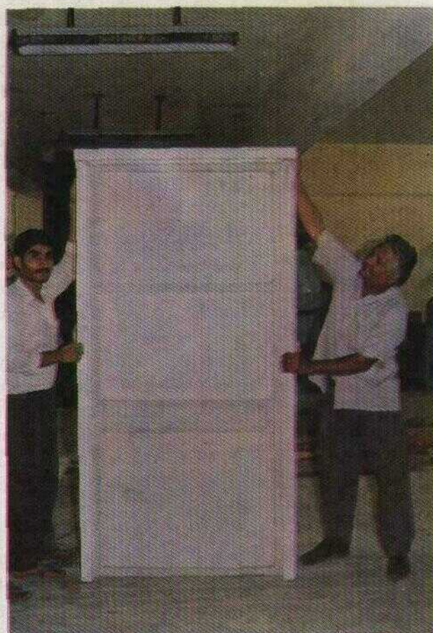
II. 7. Ferrocement Door Frame and Shutter Fitted Together
