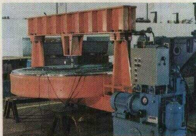
III.A.9 Helicopter Landing Grid Testing in a Special Fixture
