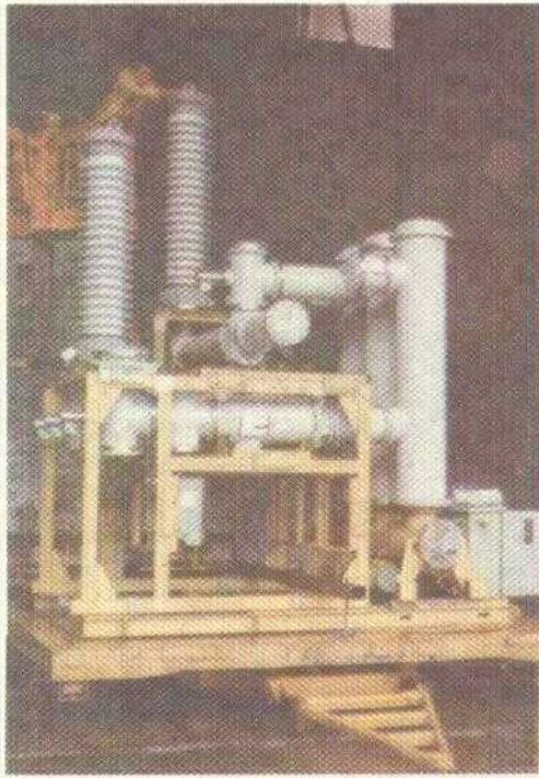
III.A.5 145 KV Gas Insulated Switchgear
