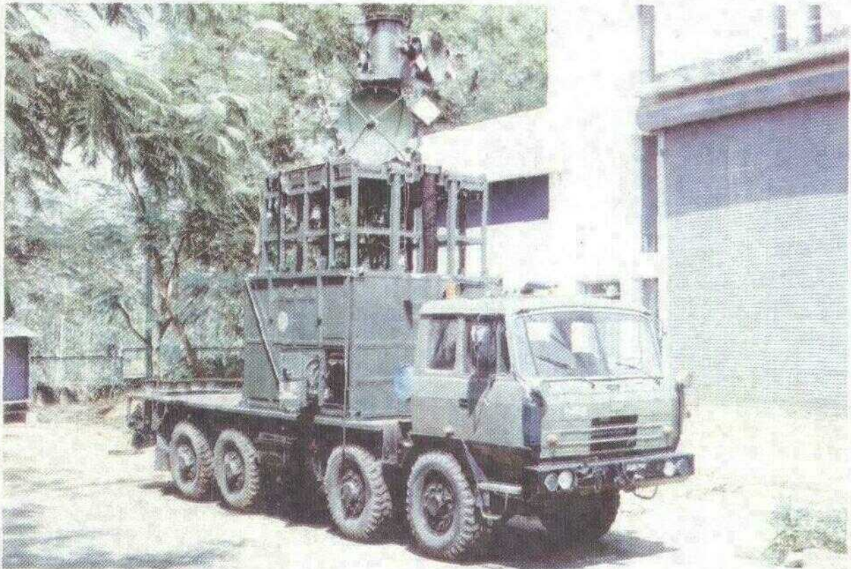
III.A.4 Sensor Retraction/Hoisting and Servo System on Wheeled Vehicle
