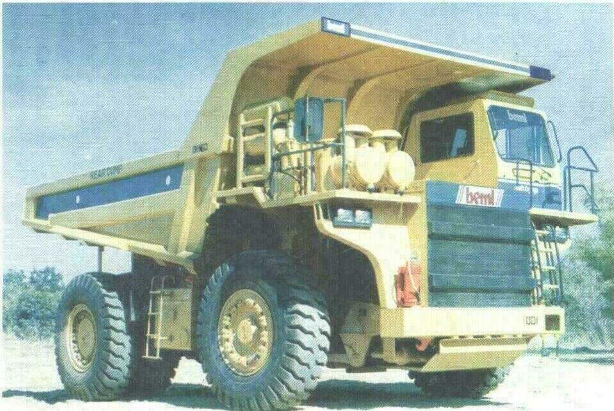
IV.7 70 ton Dump Truck developed under PATSER by M/s. Bharat Earth Movers Ltd., Bangalore
