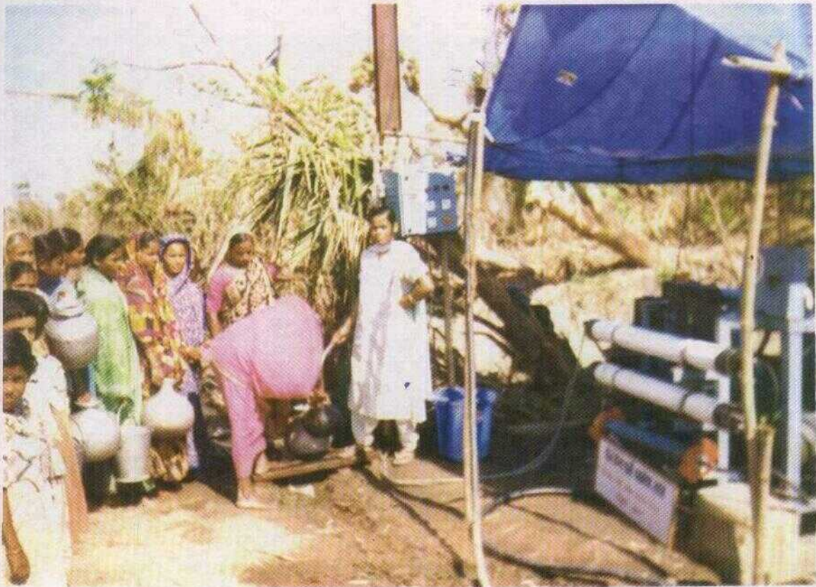
II.3 Providing safe drinking water to super cyclone affected people of Orissa at Navgaum by CSMCRI developed RO plant
