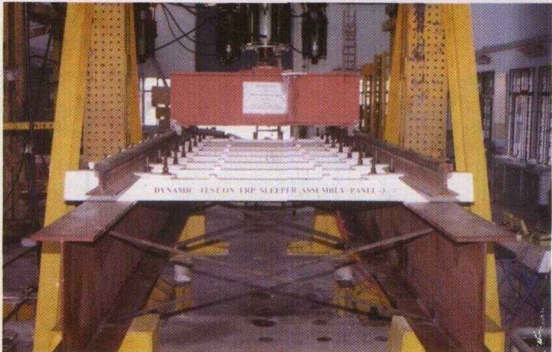
II.10 Dynamic facility for FRP sleeper testing
