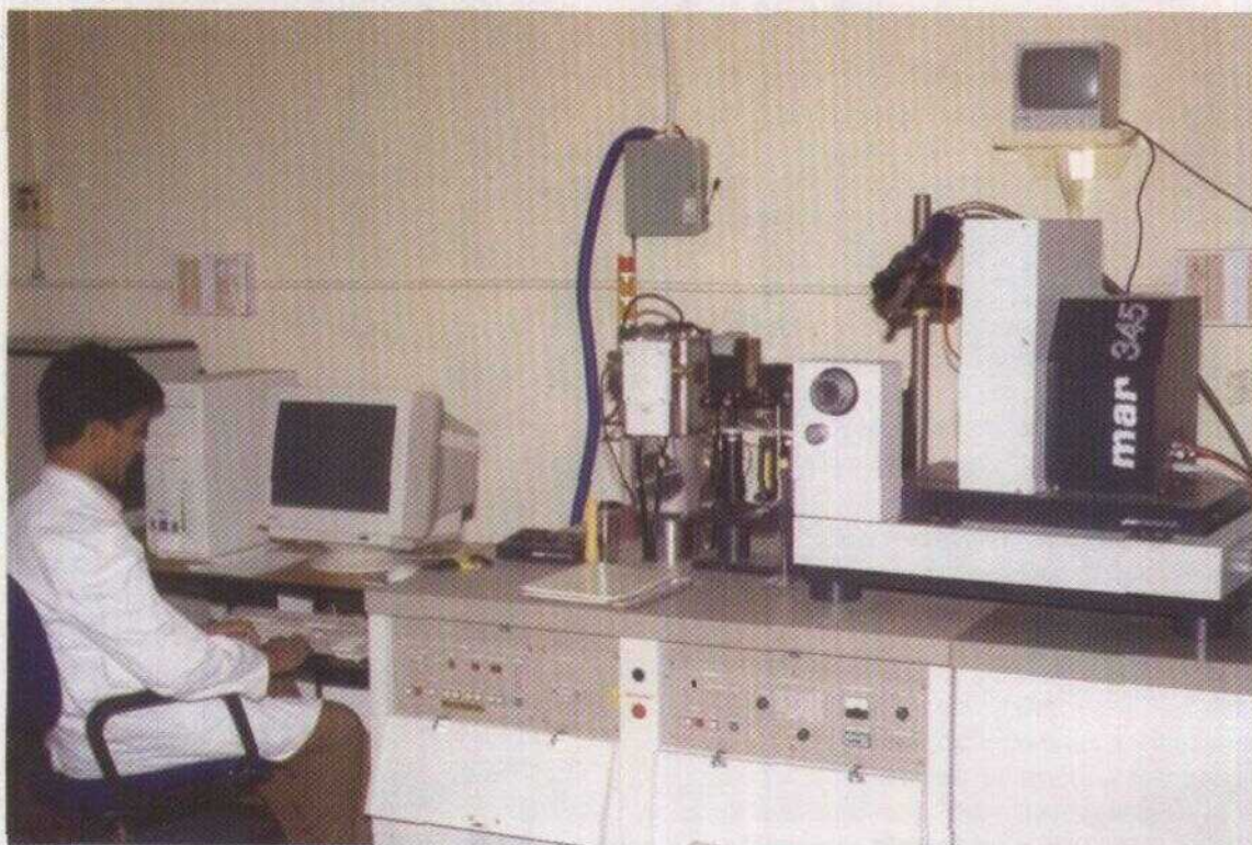
II.5 X-ray crystallography facilities set up at CDRI for structure elucidation of new molecules
