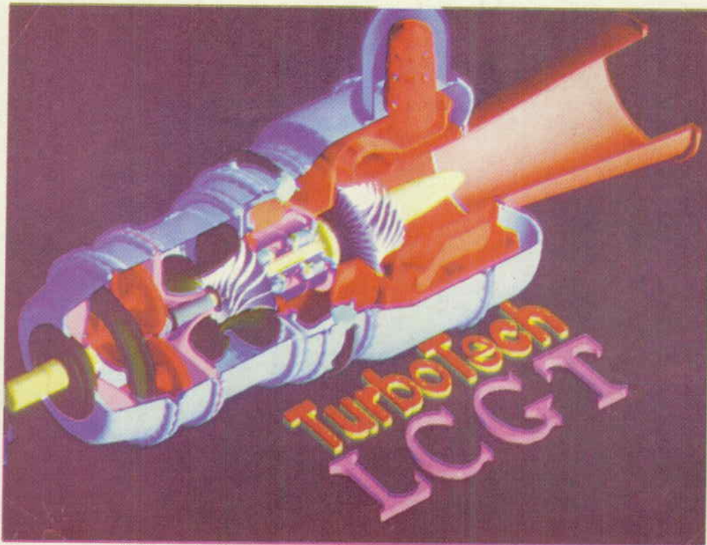
IV.2 Conceptual Drawing of Low Cost Gas Turbine under development at Turbotech Precision Engineering Pvt. Ltd., Bangalore
