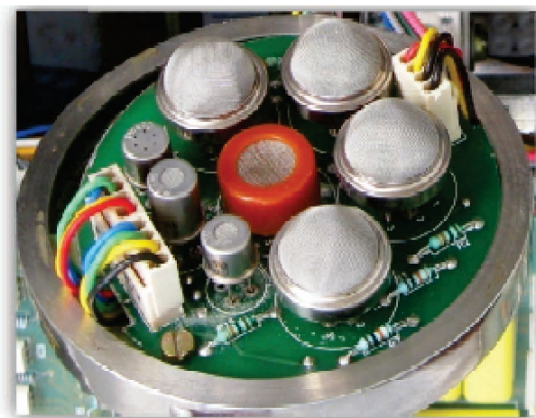
Sensor array in E-Nose developed jointly by CSIR-NEERI and CDAC-Kolkata
