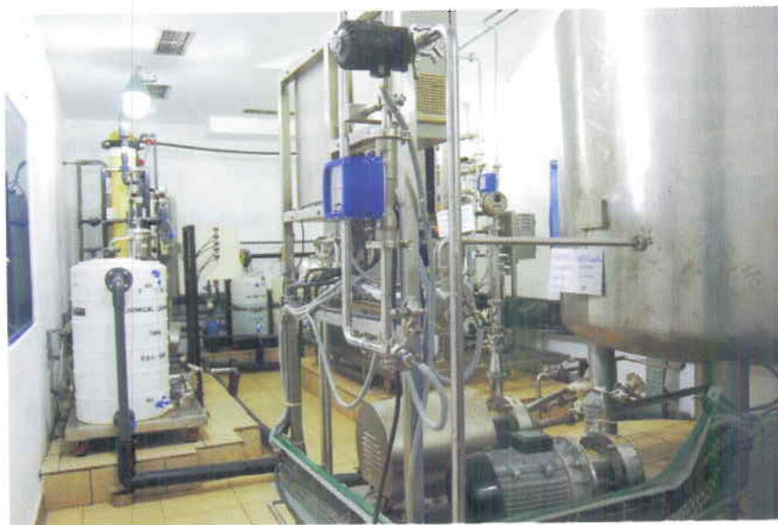
Ophthalmic Grade Purified Water System for preparation of Dorzolamide HCl
