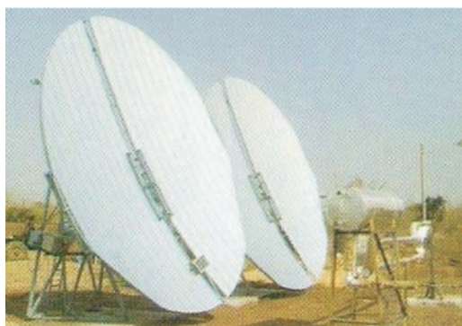
Fig 10: Hybrid System for Solar Distillation and Drying Application
