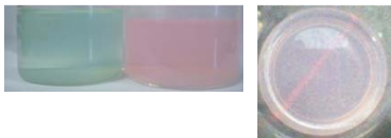
Fig 37: Laser light passing through CoAl exfoliated sample
