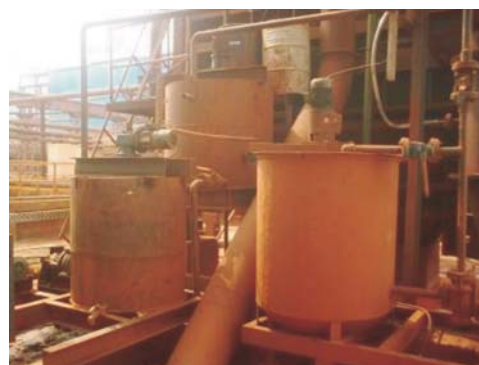
Fig 84: Conditioner and agitator with feed pump
