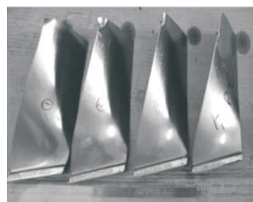
Fig 50: Tip damage to fan rotor blade (FRB-1)
