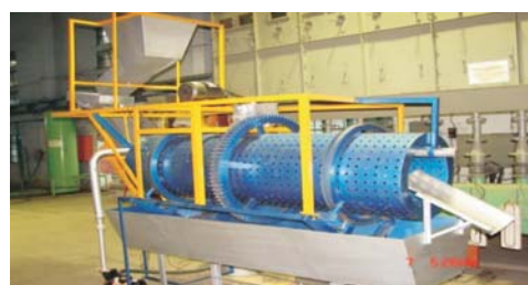
Fig 66: Washing Unit for freshly harvested ginger/turmeric
