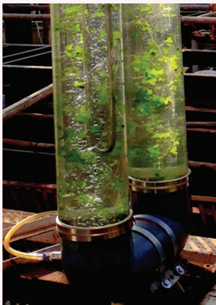
Air-lift Tubular PBRs with low power efficient sparging system
