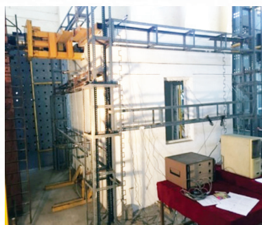
Full-scale retrofitted confined masonry building subjected to lateral cyclic load
