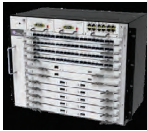
TJI-1600C platform on which the eDC card is hosted to provide eNodeB functionality
