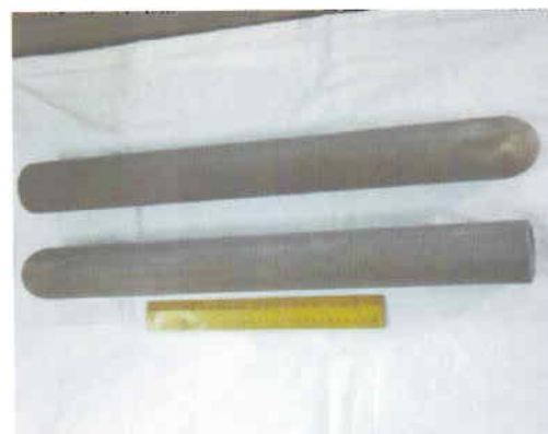
Slip cast silicon green tube of required dimensions
