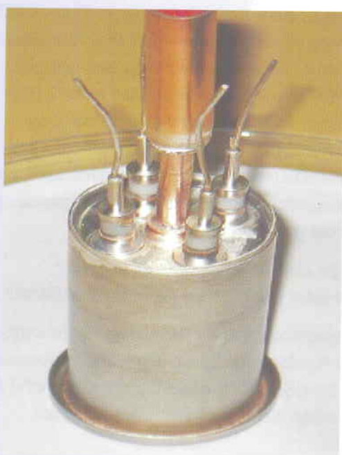
Rear view showing feedthroughs
