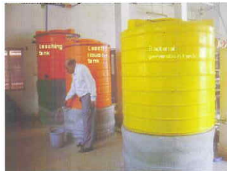
One ton capacity column for bacteria leaching of nickel from chromite ore overburden
