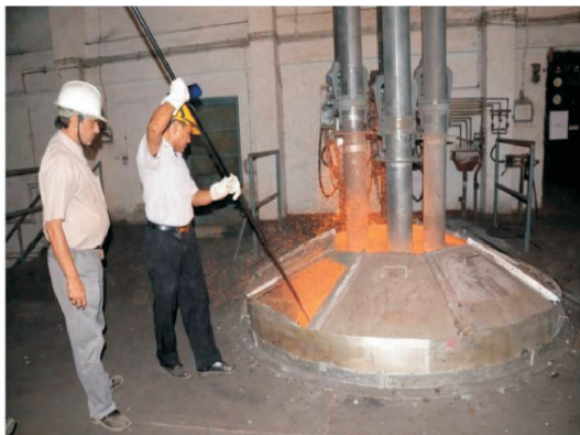
Fig. Pilot Scale submerged arc furnace operation
