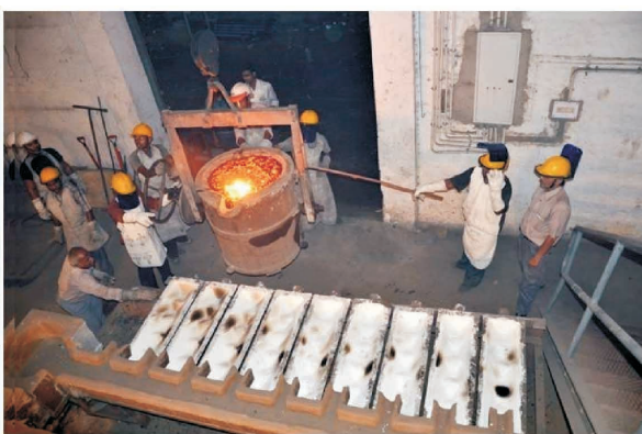
Fig. Metal tapping from submerged arc furnace
