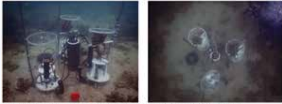
Experimental setup of the Benthic Chambers on the Seabed at Rameshwaram
