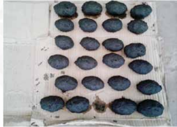
Bio-coal prepared from char of tender coconut shell
