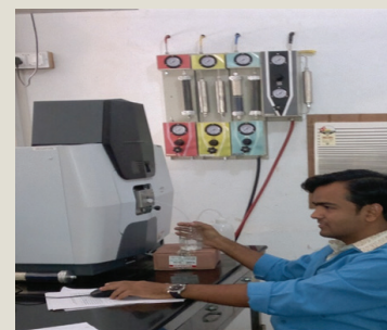
Metal Analysis using FAAS at Loyola Centre
