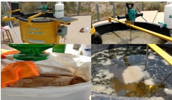
*Trail runs of AHC products of M/s Arun Industrial Products for sewage treatment at 200 L and 400 L scale at DSIR-CRTDH at IIT-Gandhinagar*
